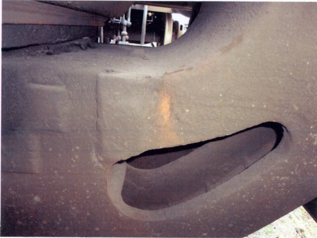
Photograph 1 – Fracture on Outer Surface of Bogie Bolster
