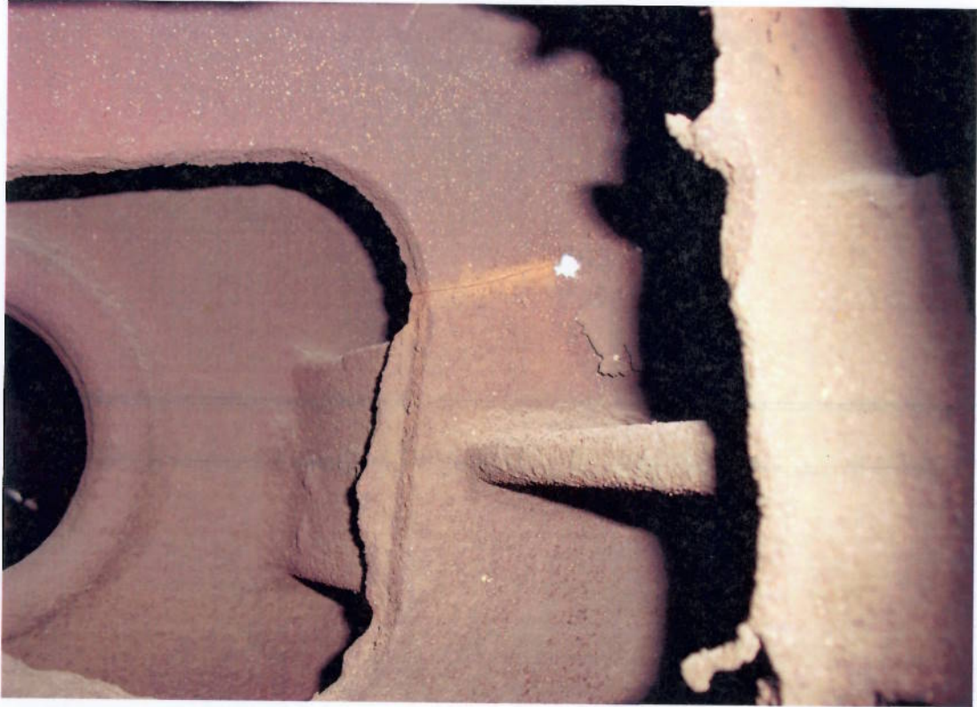
Photograph 2 – Fracture on Internal Web of Bogie Bolster
