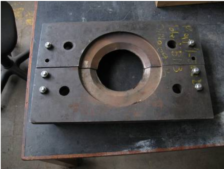
Figure 3 Full face adaptor for removing axle bearings
