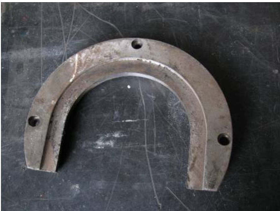
Figure 4 'Horsehoe' half adaptor for removing axle bearings
