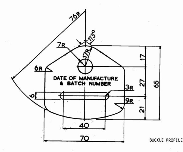
The buckles shall be free from any sharp edges, burrs etc and shall be capable of withstanding a proof load of 22 kN without failure or permanent set
